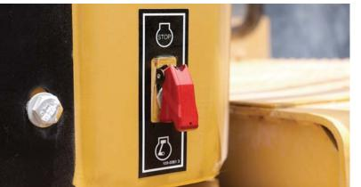
Your Cat G Series truck is designed to provide operators and technicians with easy access to common service points like engine lockout, machine system lockout, fluid level sight gauges, grease fittings and access to the engine for regularly scheduled maintenance.
