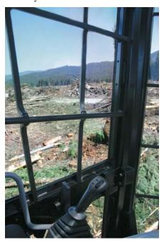
**Viewing.** Cab design optimizes post structures, and scratch-resistant polycarbonate window placement to provide excellent operator visibility to front, sides and rear. Forestry cab is designed with heavy-duty guarding, meeting all ROPS/FOPS/OPS/FOGS/TOPS and CB requirements. Windshield wipers are standard equipment on the FM cab.
