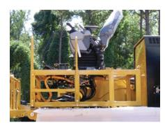
**Less-Off Cab.** A version of the 325D FM Log Loader is available less-off the cab to allow various AEM cabs to be installed by the dealer to meet regional customer needs.
