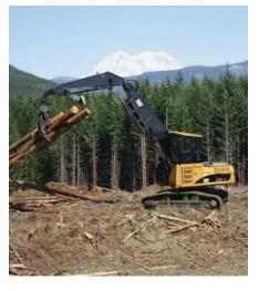
**Butt-N-Top.** The 325D FM can be shipped from the factory with an optional hydraulic arrangement and controls for AEM Butt-N-Top grapple installation, and an 11.3 m (37 ft) front.
