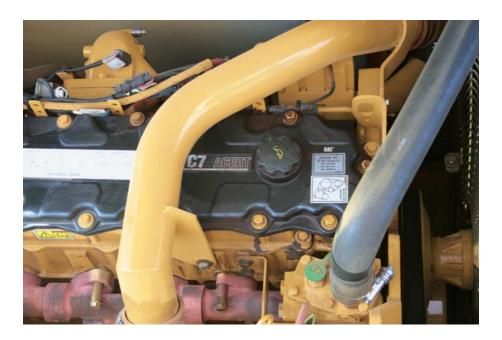
**Cat C7 ACERT<sup>TM</sup>.** The Cat® C7 with ACERT<sup>TM</sup> Technology gives the 325D FM exceptional power and fuel efficiency unmatched in the industry, and provides high performance in all forestry applications. The C7 meets U.S. EPA emissions requirements.
