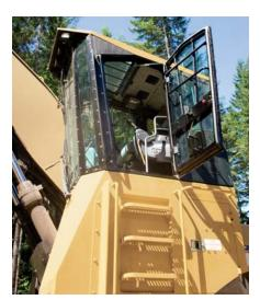
**Operator Station.** The workstation is spacious, quiet and comfortable, assuring high productivity during a long work day. Controls, joysticks and an ergonomically designed seat reduce operator fatigue.
