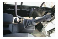
Joystick Control. Joystick controls have low lever effort and are designed to match the operator's natural wrist and arm position. The operator can operate joystick controls with an arm on the armrest and the horizontal and vertical strokes have been designed to reduce operator fatigue. Exclusive proportional control and push buttons are programmable to operator personal preferences, allowing maximum productivity.
