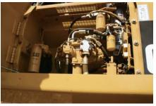
**Capsule Filter.** The hydraulic return filter, a capsule filter, is situated outside the hydraulic tank. This filter prevents contaminants from entering the system when hydraulic oil is changed and keeps the operation clean.
