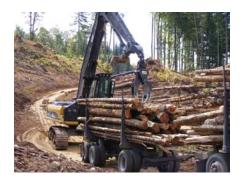
The Cat Log Loader is "Purpose Built" for Forest Applications. Completely assembled, heel-type log loaders linkage (including grapple) are available from the factory. These are well suited to loading, shovel logging and millyard applications.
