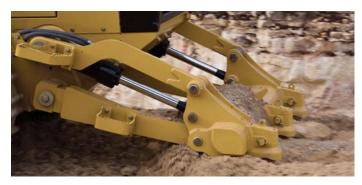
Ripper – A 3-shank parallelogram ripper facilitates
