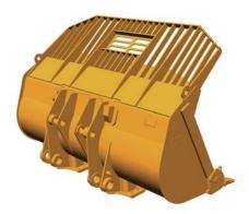
• General Purpose Landfill bucket – has a capacity of 4.9 m<sup>3</sup> (6.4 yd<sup>3</sup>) and can be equipped with an optional trash rack for dozing lightweight materials. This bucket is designed for easy loading in stockpile or hard bank materials. Adding the trash rack helps prevent material from spilling over the top and increases dozing capacity by 52%.
