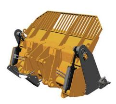
• Multi Purpose Landfill bucket – has a capacity of 4.6 m<sup>3</sup> (6.0 yd<sup>3</sup>) and can greatly expand the 973D's versatility. It can act as a typical bucket for loading trucks, dozing waste or digging. It can also instantly change into a dozer-type blade for spreading cover material, or it can sort material with the ability to clamp on to debris. By adding the trash rack to this bucket, its capacity to doze and load material increased 53%.
