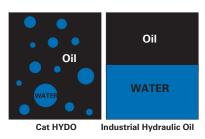
Typical industrial hydraulic oils separate water and oil, which can cause valve sticking or excessive wear on your hydraulic system. Cat HYDO disperses small amounts of water throughout the oil to ensure proper lubrication.
