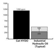
Caterpillar recommends a minimum of 900 ppm zinc for protecting pumps, motors and valves from excessive wear. Cat HYDO contains more than twice as much zinc as typical Anti-Wear industrial hydraulic oil to maximize your hydraulic system's life and performance.
