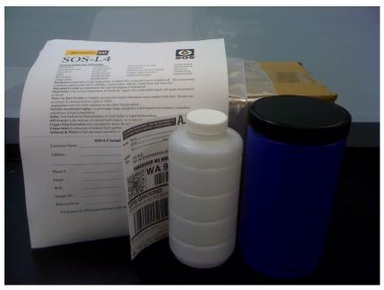
The SOS-CSA is intended to give you a spot check for the most common problems caused by storing the fuel. The fuel will be tested for Water/Sediment and microbial growth. This package is designed for any industry that has onsite fuel storage such as hospitals, banks, critical data centers, etc. This is also a great starting point for customers that are experiencing filter plugging in their fuel system or poor machine performance.
