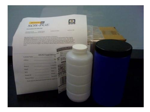
The SOS-PGE package is great in determining the amount of contamination present in your fuel. This package was designed in accordance with PGE specifications for fuel quality at their facilities. This package covers the particulate contamination level of the fuel as well as water and microbial growth in your fuel.
