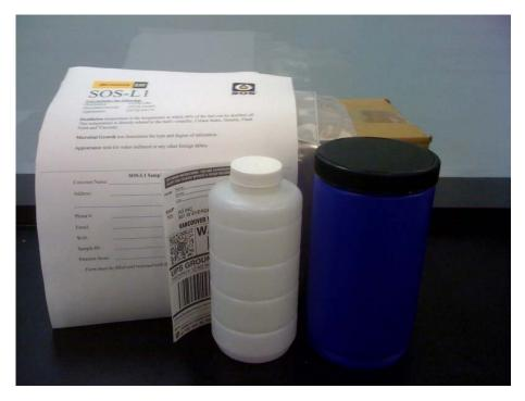
The SOS-L1 package is a great starting point in checking the life of your fuel. This basic package is designed to detect any foreign contaminants present in the fuel, from lighterend to heavier-end petroleum products, to microbial growth and visible water and sediment.
