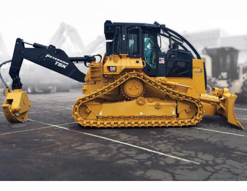
Engine Model: Gross Power: Cat® C7.1 Tier 4 Final 202 HP @ 2,200 RPM
