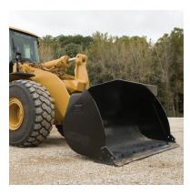
The Caterpillar Fusion Coupler System includes a full line of buckets for use in a wide range of job site situations.
