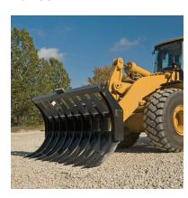
Loader Rakes are durable, high-capacity tools for land clearing and site clean up. Rakes are available with single or dual top clamps.
