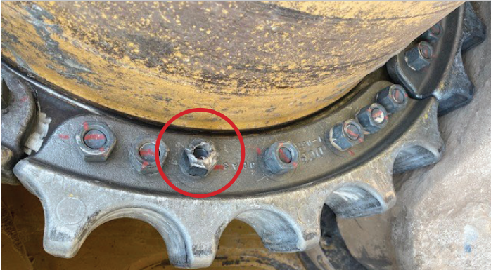
Trek (DCF) bolts became loose from wear.
