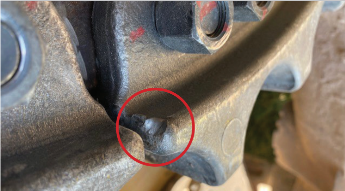
Trek (DCF) segments hit each other, loosening them over time.
