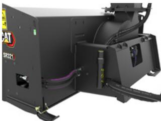
Tool mounted and sealed from the elements, this document holder includes all the operation manuals and maintenance guides required for proper operation of the tool.
