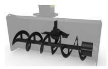
Two-stage design uses auger and impeller to move a greater capacity of snow quickly and efficiently. Auger and impeller are reversible which allows the operator to expel obstructions without exiting the machine.
