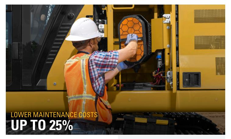
With synchronized and extended maintenance intervals, you get more done at a lower cost compared to the 330F. Consolidated filter locations make service faster. Hydraulic, air, and fuel tank filters have increased capacity and longer life. Access to the operation and maintenance manual is easy through the in-cab monitor.
