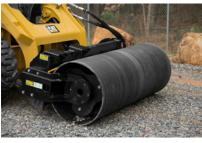
HIGH STRENGTH STEEL DRUM Durable high-strength steel drums are roll formed and finish welded for a smoother surface and longer life.
