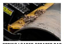
Spring-loaded dual direction non-metallic scraper bar maintains constant pressure on drum to prevent material build up. Non-metallic design minimizes noise.
