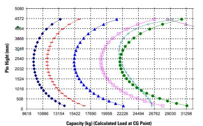
NOTE: Static tipping loads and operating weight are based on the following loader configuration: L3 Michelin XHA Tires, Air Conditioning, Ride Control, Powertrain Guard, Full Fluids, Fuel Tank, Coolant, Lubricants, and Operator.
