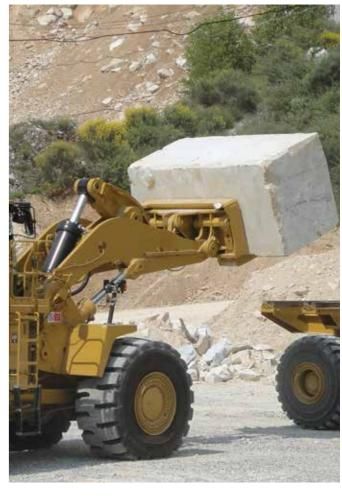
Block Handling Work Tools are extreme duty tools built for the demanding quarry and block-handling markets. The complete system is based around a quick coupler and a series of rugged tools specifically for handling and manipulating large stone blocks. These tools are designed to withstand the demanding and harsh environment of block handling applications. Various work tools are available to assist operators in all block handling applications.
