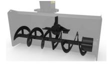
Two-stage design uses auger and impeller to move a greater capacity of snow quickly and efficiently. Auger and impeller are reversible which allows the operator to expel obstructions without exiting the machine.
