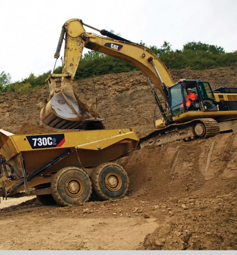
The Cat 730C2, with a 17 m<sup>3</sup> (23 yd<sup>3</sup>) 28 tonnes (31 tons) capacity, offers demonstrated reliability and durability, high performance and productivity, superior operator comfort and lower operating costs.
