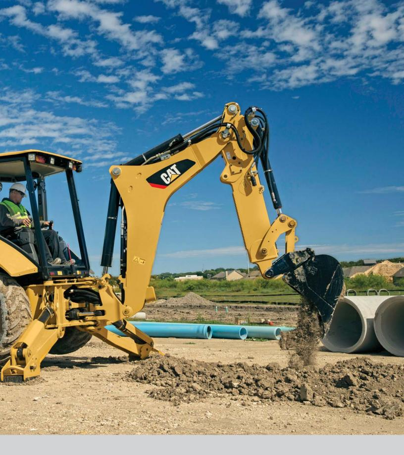
Experience the Backhoe Loader designed around customer feedback. The Cat 420F2 Backhoe Loader puts all the machine controls at the operator's fingertips. Operate all auxiliary controls with thumb rollers. Move from job site to job site quickly and smoothly with the additional 6th gear on the autoshift transmission and optional lock-up torque converter.
