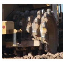
**Cleaner Bars.** Help keep the drums free of carry-over dirt regardless of rolling direction. A pass-through bolt design allows for easier serviceability.
