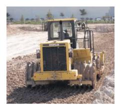
Compaction. Is achieved from the bottom of the lift to the top. The tapered pads walk out of the lift without "fluffing" the soil. The top of the lift is compacted and the surface is relatively smooth and sealed so hauling units are able to maintain a high speed when traveling over the fill. 815F Series 2 travel speed allows for four forces of compaction: pressure, manipulation, impact and vibration. Since it can also spread fill, the number of spreader tractors may be able to be reduced.
