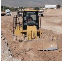
**Applications.** The 815F Series 2 excels at compacting, spreading fill, backfilling and boosting scrapers. With the ability to work at higher speeds over other types of soil compactors, the 815F Series 2 can keep up with a fast-moving scraper fleet or an articulated truck hauling operation. When speed and dozing capability are required job duties for a soil compactor, the 815F Series 2 has no equal.
