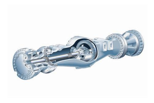
**Front Axle.** Is rigidly mounted to the frame to support the weight of the compactor, internal torque loads and external loads applied during compacting and dozing operations.
