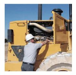
**Right Side Service Access.** Puts the the fuel filter and water separator, fuel primer and engine oil dipstick within easy reach.
