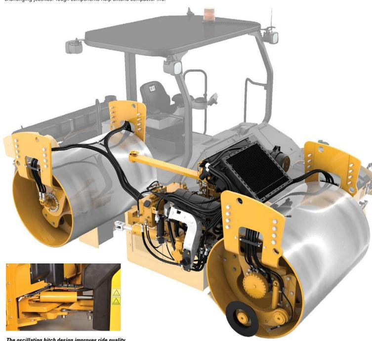
The oscillating hitch design improves ride quality on uneven terrain.
