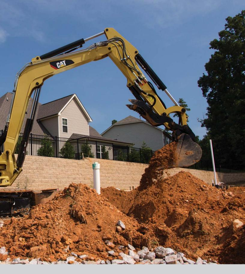
The Cat E2 Series Mini Hydraulic Excavators are designed to carry on the solid performance of their E Series predecessors, while adding even greater value for the customer. The new High Definition Hydraulic (HDH) System, redesigned operator station and enhanced digital control panel specially designed for Cat Mini Excavators – COMPASS (Complete, Operation, Maintenance, Performance And Security System) – are all standard features that improve performance and increase value.
