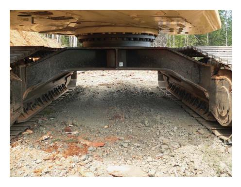
**Heavy-Duty Top Rollers.** Track rollers with dual supports replace standard single post mounted carrier rollers to assure superior endurance.
