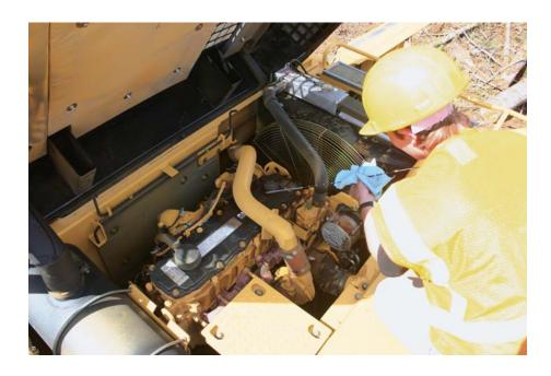
**Ground Level Service.** The design and layout of the 324D FM was made with the service technician in mind. Many service locations are easily accessible at ground level allowing critical maintenance to get done quickly and efficiently.
