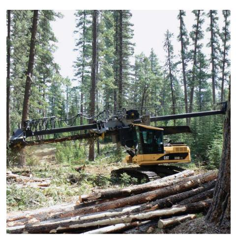
**Cat Roadbuilders.** A General Forestry model can be configured as a Cat Roadbuilder and can be equipped with bucket, thumb, clamshell or clearing grapple to fit a wide range of forest road jobs.
