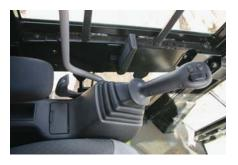
Joystick Control. Joystick controls have low lever effort and are designed to match the operator's natural wrist and arm position. The operator can operate joystick controls with an arm on the armrest and the horizontal and vertical strokes have been designed to reduce operator fatigue. Exclusive proportional control and push buttons are programmable to operator personal preferences, allowing maximum productivity.
