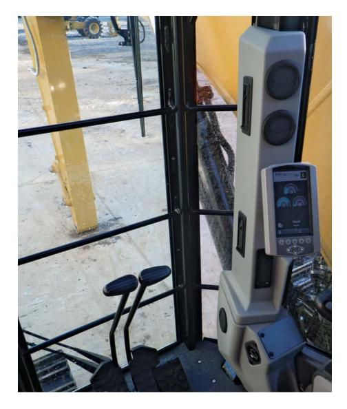
Climate Control. Positive filtered ventilation, a pressurized cab with bi-level air conditioner, heater and defroster keep operator comfortable in all types of weather conditions. Cab also has a forced air fan and a large fresh air window.
