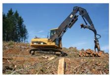
**Pilot System.** The pilot pump is independent from the main pumps and controls the front linkage, swing and travel operations.
