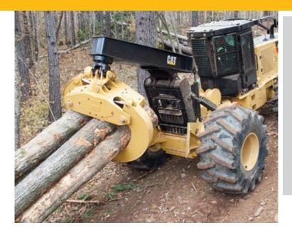
Box-section construction was used in the arch and boom designs to transfer heavy loads efficiently into the main frames. The arch gate is integrated into the arch and comes with a bolt-on fairlead roller assembly for skidders ordered with a winch, or a bolt-on guard, for skidders not equipped with a winch.
