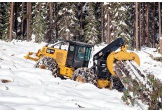
Power to the ground is an advantage of the Cat D Series. The axles are designed specifically for the skidder application and the gear ratios cause the power to be generated in the axles reducing torque in the transmission and drivelines extending their life. Both drawbar performance and durability are improved.
