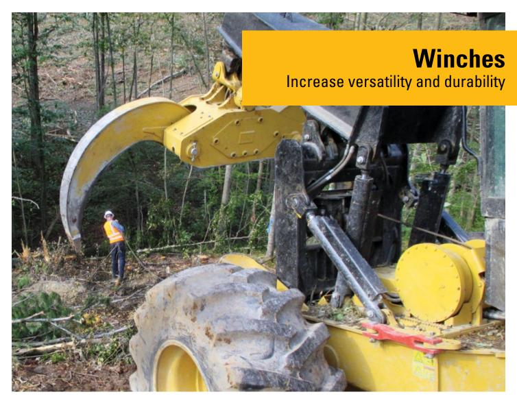
Logging and retrieval winches are available as options. Both are hydraulically driven, have the same pulling power and feature friction style clutches for increased durability and functionality. Both the retrieval and logging winches are operated by a joystick for more control over the reeling speed.
