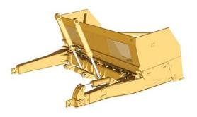
Both scoops come with dual lift cylinders for increased lift capacity. Integrated stabilizer system makes sure that the scoop stays stable and centralized on the machine. Scoop tilt function is standard and provides  $\pm 15$  degrees of tilt to maintain grade conditions and keep your operation safe.
