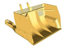
Large capacity scoops for both wood chip and coal applications. A mesh screen integrated into the back of the scoop maintains visibility to the cutting edge. The chip scoop version has extra screens at the top due to higher capacity.
