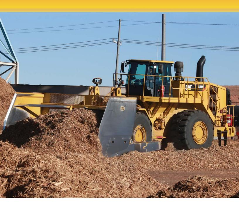
Engine Model Cat® C18 ACERT™ Emissions U.S. EPA Tier 4 Final/EU Stage IV, Tier 3 Equivalent, or Tier 2 Equivalent Gross - SAE J1349 419 kW 562 hp Net - SAE J1349 370 kW 496 hp
