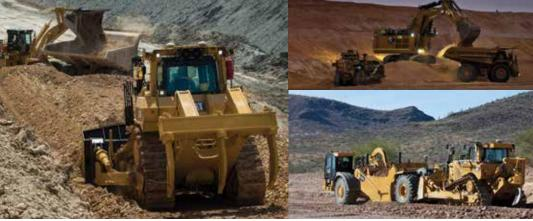
Versatile Cat dozers keep mine sites operating at peak productivity and are essential machines for dozens of jobs, such as truck dump and site maintenance, leveling the bench after blasting, establishing a general gradient and width for the bench, and working alongside loaders, shovels and draglines to support the performance of the loading and hauling fleet.
