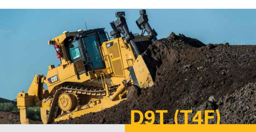
With its robust durability and high availability, the D9T will help you get more done at the lowest cost per unit of material moved. Because of its size, it makes a great utility machine at a mine and is useful for removing overburden or in mine reclamation. The D9T also works well in loose or blasted material. The D9T can easily move around on a mine site, performing tasks such as truck dump maintenance, ripping, stripping, road building, stockpile management, dragline support and trapping.
