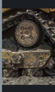
Cat dozers have an elevated sprocket and fully suspended undercarriage, which work together to provide increased traction and a smoother ride in addition to improved production and longer component life.
