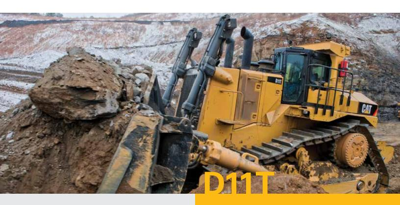
The D11T is a highly effective mass dozing machine purpose-built to move large quantities of material long distances. Its reliable engine delivers the power and high productivity you demand, with exceptional service life. This machine is ideal for removing overburden or in mine reclamation, working efficiently to move loose or blasted material.
