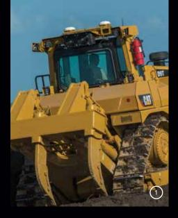
1. Cat Grade Control 3D uses dual ROPS mounted GNSS antennas and in-cylinder position sensors to provide precise positioning of the cutting edge, eliminating the need for masts and cables on the blade. The system also reduces the need for grade staking and grade checking; as a result, fewer people are required on the job site, which lowers personnel costs and enhances safety.
