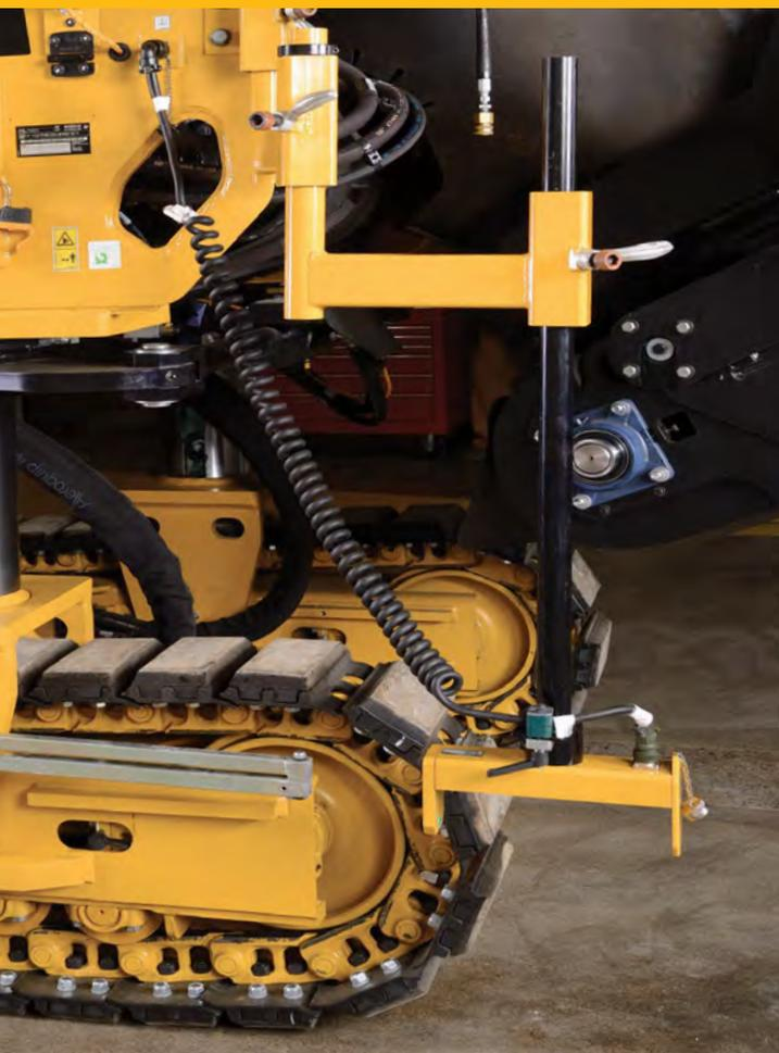
*Each sensor has five transducers; the high and low readings are discarded and the remaining three are averaged for a true average reading.*
