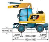
Roading position with 2450 mm (8'0") stick Maximum boom height in roading position with a VA is below 4 m (13'1")
