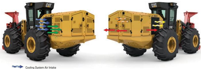
Engine/Hydraulic Compartment Air Intake - Electric reversing fan pressurizes the engine/hydraulic compartment with cool ambient air
