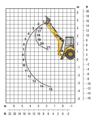
Lift Capacities are over-end values. Machine equipped with 4WD, OROPS, 0.76 m³ (1.00 yd³) general purpose bucket and no counterweight. Extendible stick includes 460 kg (1,015 lb) counterweight.
