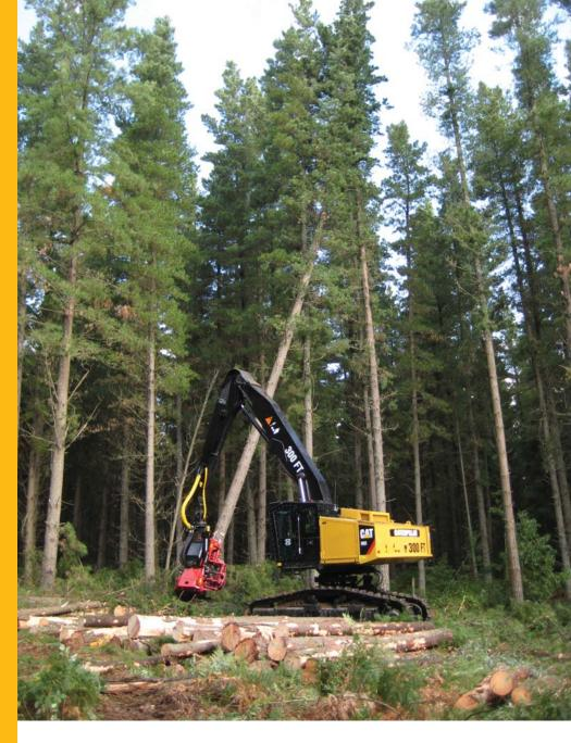
The Series 2 track feller bunchers feature smoother hydraulic performance, better fuel economy, a more comfortable operator station and better visibility. Both the Cat® 541 Series 2 and the 552 Series 2 are full tail swing machines designed for high production clear cut and for clear or select cut in rough terrain. The 552 Series 2 is a leveling machine for more comfort on steep terrain.
