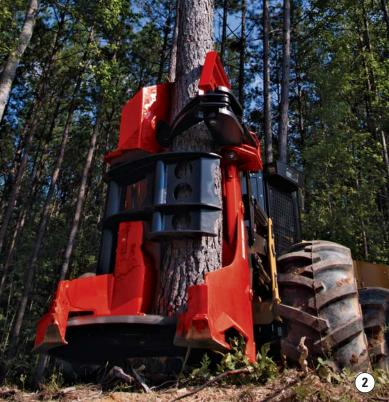
New work tools have been developed to meet the increased capabilities of the C Series wheel feller bunchers, including the new SH-56B, the most versatile and balanced high capacity bunching saw in the market.
