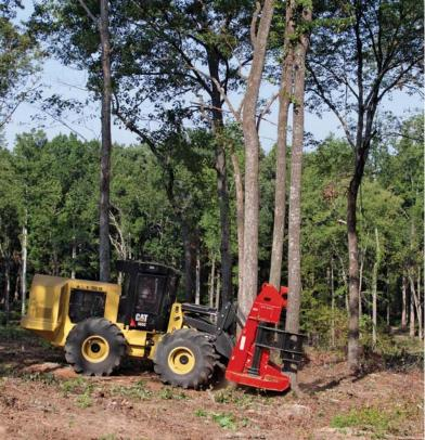
Unique operating modes, combined with complete electrohydraulic controls, provide the operator with a smoother machine with increased productivity. These modes include Terrain Selection Mode to optimize performance on hills or flat ground, Creep Mode to improve machine functionality, particularly in first thinnings, and Road Steer Mode for high-speed transport of the machine.
