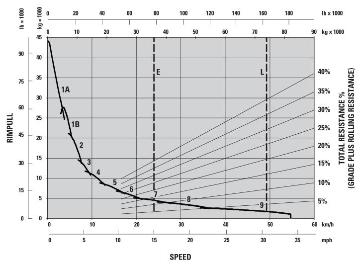
1A – 1st Gear (Converter Drive)
