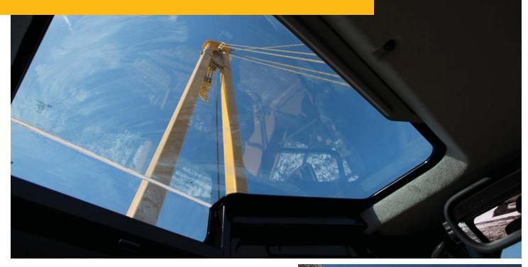
The new, optional enclosed cab is designed by Caterpillar specifically for demanding pipeline applications. The cab height meets shipping requirements and may be shipped by truck without removing the cab and Rollover Protective Structure (ROPS). The cab is fully sealed, filtered, and pressurized for harsh environments.
