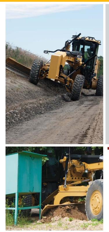
If you work in soft underfoot conditions where traction can be a challenge, optional All Wheel Drive (AWD) can give you the additional power to the ground you need to work more efficiently in mud, gravel, sand or snow. The added traction helps reduce sliding on side slopes.
