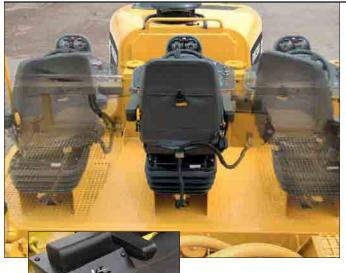
**Hydraulically-assisted sliding platform.** The operator can position the platform to any desired position to provide clear, all-around visibility to both sides of the machine. Platform can be accessed from either side of the machine.
