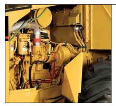
Daily service points are accessible from ground level and are grouped on one side of the engine. Hinged ground level side panels open wide for total access to engine components. Lower side panels can easily be removed for even greater access.
