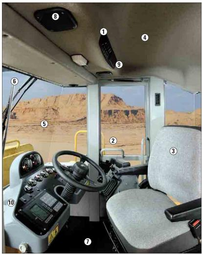
**Pressurized iso-mounted cab.** Maintains noise, dust and the elements out, and comfort in.
