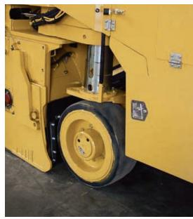
Flush Cutting Capability Wheel undercarriage option shown.
