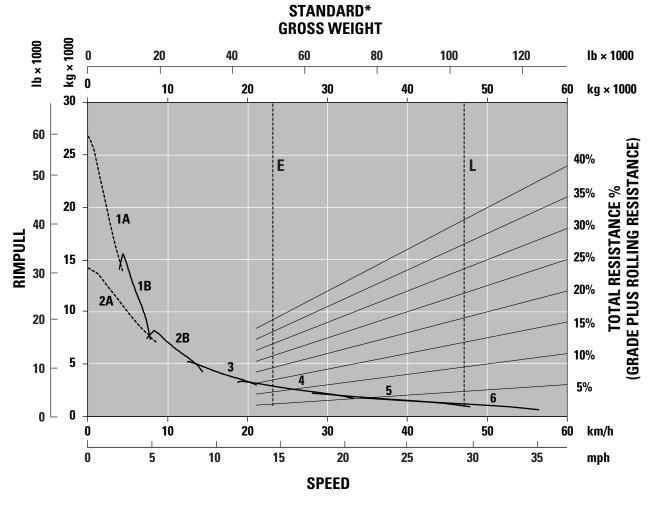
1A – 1st Gear (Converter Drive) 1B – 1st Gear (Direct Drive) 2A – 2nd Gear (Converter Drive)
